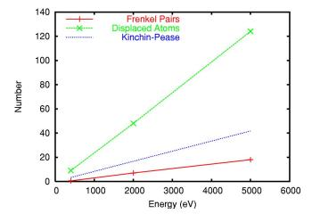
FIG. 7. (Color online) The number of defects and displaced atoms as a function of PKA energy. The displacement energy threshold for the Kinchin-Pease formula was taken as  $E_D$ =60 eV. The lines are guides for the eye.
