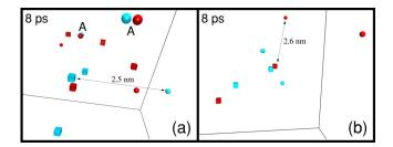
FIG. 5. (Color online) Examples of the spread-out residual damage after the collisional phase of the cascade at 2 keV. (a) The image shows three separated Mg vacancies and four O vacancies. There are two MgO di-interstitials (labeled A), one Mg interstitial, and two O interstitials. (b) In this case, only well-separated monointerstitials and vacancies occur.
